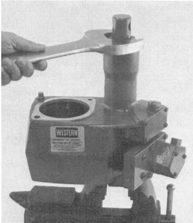
Step 4: Remove packing nut, packing set, and plunger assembly from the lift cylinder housing. Turn packing nut counter-clockwise.
