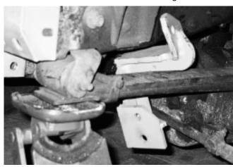
2. Using the top two holes, loosely attach the front of the mount to the cross mount using the supplied 5/8" x 1-1/2" cap screws and 5/8" locknuts. Repeat on other side.
