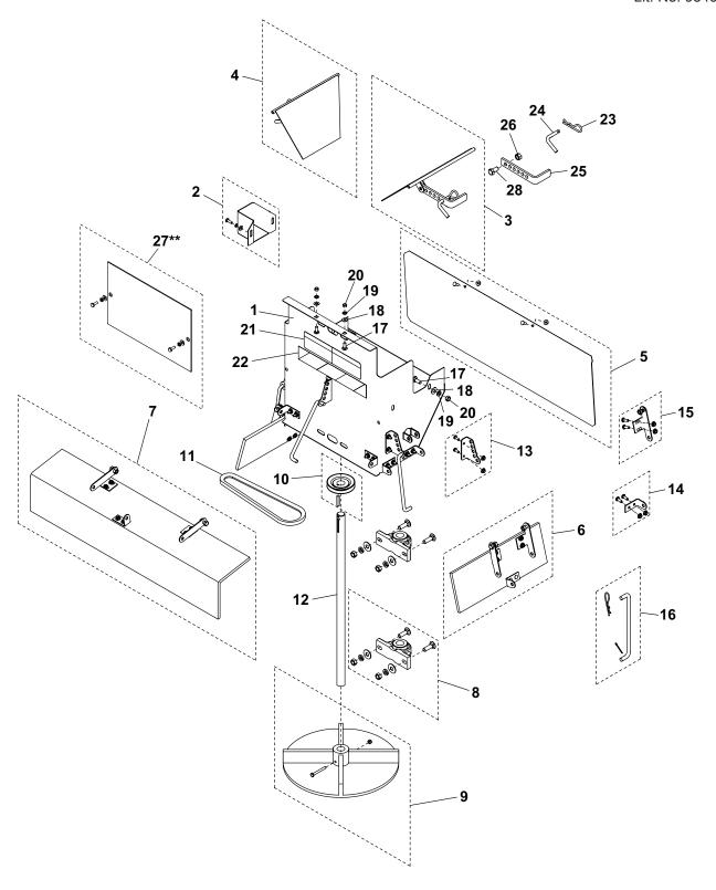
This parts list is for FISHER® PRO-CASTER Hopper Spreaders with serial numbers 0303 and higher.
