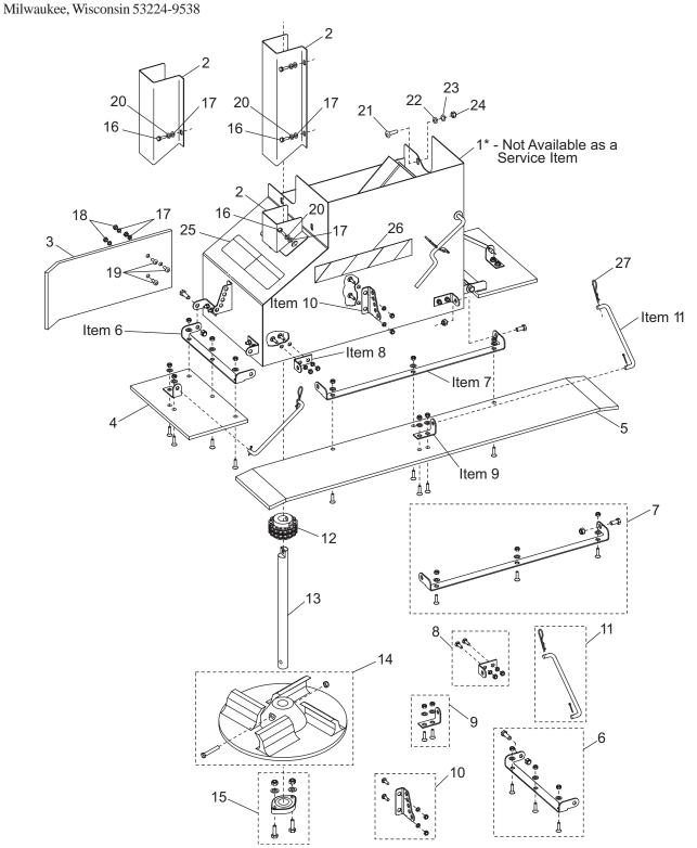
This parts list is for WESTERN<sup>®</sup> ICE BREAKER<sup>™</sup> Hopper Spreaders with serial numbers 0126 and higher.
