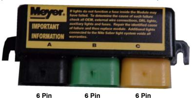
07347 Rev 2 (with replaceable fuses) requires new "B" harness 07609 when replacing 07116 modules. (07609 included with 07548 kit)
