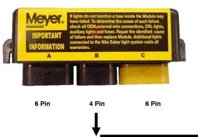
07347 original (with non replaceable fuses) requires new "B" harness 07609 when replacing 07116 modules. (07609 included with 07548 kit)
