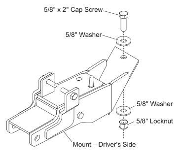
NOTE: The cap screws and washers can be placed by passing them through the opening just under the lower A-arm first and then positioning them in place at the cross member hole.
