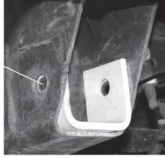
3. Beginning with one mount, align the forward mount holes with holes in the frame. Insert two 1/2" cap screws through the forwardmost holes and fasten loosely with flat washers and locknuts. Insert one 1/2" cap screw up through the mount and bottom of the frame. If necessary, ream the vehicle frame using the rear mount slot as a guide. Use a washer on both the mount and nut side.
