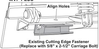
**WIDE-OUT™:** Determine which holes will be used to install the shoe bracket. The inside front slot should line up with an existing cutting fastener. The top slot to the outside of the bracket should line up with the outside hole in the shoe mounting bracket.
