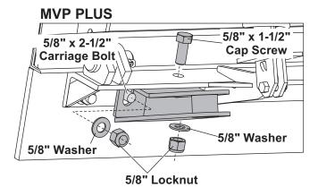
WIDE-OUT™: Insert a 5/8" x 1-1/2" cap screw through the outside top hole of the shoe mounting bracket and shoe bracket. Attach a 5/8" washer and locknut to the cap screw and hand tighten.
