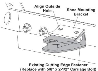
2. Replace the existing locknut and cutting edge fastener with a 5/8" x 2-1/2" carriage bolt, then position the shoe bracket against the rear of the base angle.
