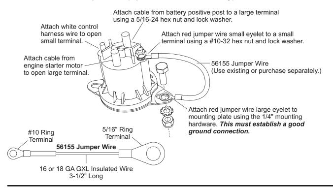
NOTE: Overtightening terminal attaching nuts may cause seal failure, resulting in premature failure of this relay.
