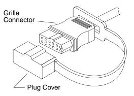
Find a convenient location in the grille, on the battery side, for the battery cable. Slide the grille plate onto the plug. Attach the grille plate to the grille with cable ties.
