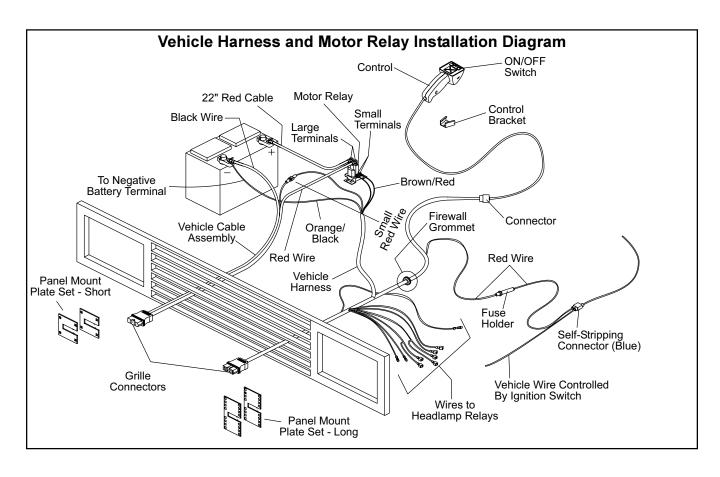
9. Attach the red wire from the vehicle cable to one of the large terminals on the motor relay. Secure with a lock washer and 5/16" jam nut.
