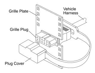
8. Route the vehicle cable through the grille at the selected location and through or around the radiator bulkhead to the motor relay. Be sure to avoid sharp edges and hot or moving parts.
