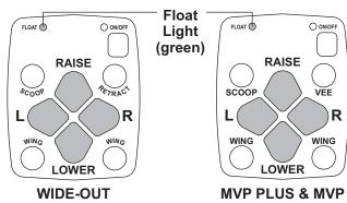
The four diamond-shaped buttons in the center of the control face, when pressed, will result in the following blade movements:
