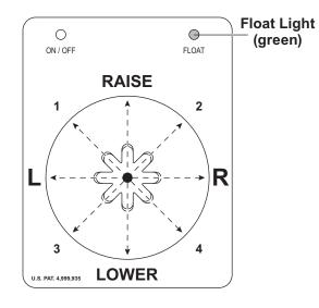
From the center position, the control lever can be moved in one of eight (8) directions to control various movements of the snowplow blade. To change from one movement of the blade to another, the control lever must be moved back to the center position before selecting the desired function. Whenever the lever is released, it should spring back into the center position to stop any blade movement.
