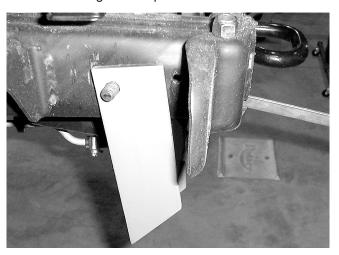
Insert a 1/2" cap screw with handle into the truck frame. Place a washer onto the cap screw, then insert the cap screw down through the bottom frame slot and the front mount. Place a washer and 1/2" locknut on the cap screw and hand tighten. Repeat on other side.
