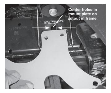
3. Mark the centers of the two holes on the frame and remove the mount plate.
