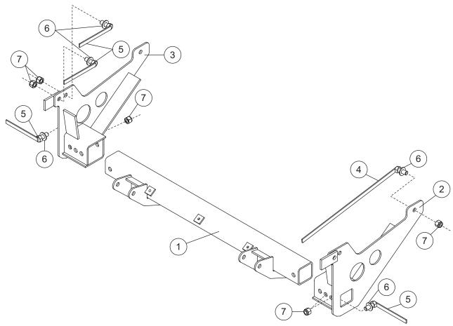
Outermost holes used for Dakota, middle holes for Durango applications.
