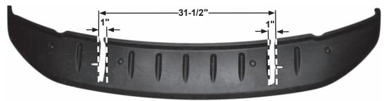
Cut slots in air dam as shown.
