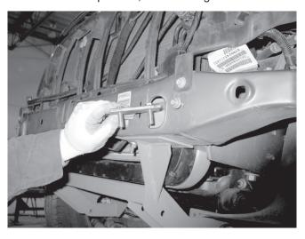
11. Insert a 3/8" flat washer through the square hole in the front cross member and position it over the round hole located just to the side of this. Bend a 3/8" cap screw with handle as needed to insert it through the square hole and hook it down through the 3/8" flat washer, through the front cross member, and through the slot in the plow mount. Place a 3/8" flat washer and a 3/8" locknut on the cap screw, and hand tighten.
