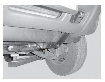
25. The end pieces of the air dam are fastened to both the bumper and the plastic wheel-well using two plastic rivets as shown. This procedure requires the use of a Marson brand Klik-Loc<sup>™</sup> plastic rivet setter number 48000 or equivalent, which is available from many local automotive centers or dealerships.
