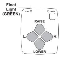
The four diamond-shaped buttons in the center of the control face, when pressed, will result in the following blade movements:
