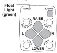
The four diamond-shaped buttons in the center of the control face, when pressed, will result in the following blade movements:
