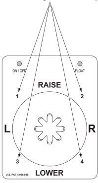
The security equipped controls can be identified by the numbers one through four on the faceplate of the control, as shown above. The isolation module for the snowplow must also be equipped with SECURITY GUARD system programming. POWER HITCH 2 hydraulic units with serial numbers beginning with 09061610 and later have the SECURITY GUARD system programming. SECURITY GUARD system enabled modules can also be identified by the dash three (-3) after the model number on the module itself.
