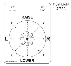
Moving the control lever in straight lines up and down or from side to side on the control body will result in the blade movements described in the following tables.
