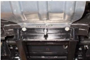
Note: Before tightening the fasteners, the Clevis Frame (\*) should be level with the ground and pushed back as far under the vehicle as possible.
