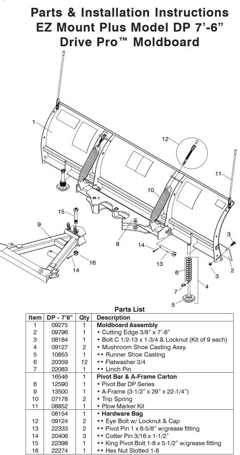
Parts indented are included in the assembly under which they are indented.
