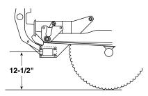
The recommended push beam height for this undercarriage assembly is  $12-1/2^{\text{m}}$  from the center of the push beam to level ground. DO NOT exceed 14-1/2<sup>n</sup> in height for this undercarriage.
