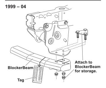
7. Level the pushbeam with the floor and torque the hanger plate hardware, making sure that the first hole in each hanger plate is aligned with the flat surface in the frame.
