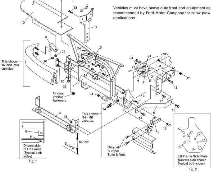
**WARNING:** This mounting is not designed for installation on Ford Bronco and F-150 vehicles with 1-A stabilizer bar. (Part of handling package option on vehicles with 3550 lb. front suspension).
