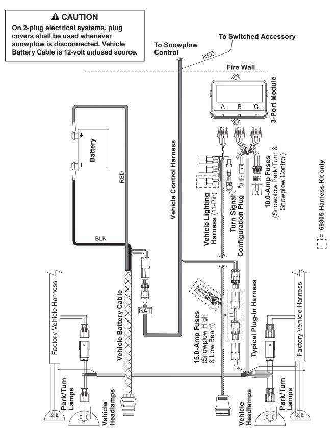
TYPICAL 3-PLUG, 3-PORT MODULE SYSTEM DIAGRAM
