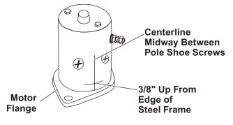
4. Use a file or grinder to create a minimum of 5/16" wide x 3/4" high flat spot centered on the center punch mark. Make sure that all paint is removed in the area covered by the ground cable terminal when it is attached.
