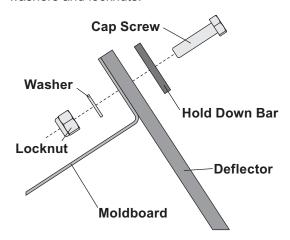
4. Secure the deflector with the remaining hold-down bars and fasteners, aligning them as shown below. When more than two holes are available in the hold-down bar, use the outermost holes.
