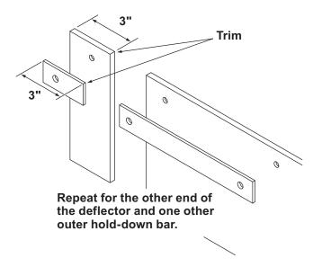
3. Align the center hole in the deflector with the center hole in the top of the moldboard. Place the center hold-down bar on top of the deflector, making sure the center holes are aligned, and secure with three 5/16" x 1-1/4" cap screws, washers and locknuts.
