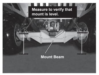
Measure the distance between the mount beam rear hole and the ground. If it exceeds 11-1/2", install the accessory Height Adapter Plate Kit (PN 77555) to ensure optimum plowing performance.
