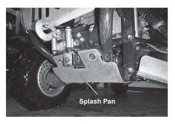
2. Position two U-bolts over each frame rail. Position the skid pan assembly in place against the bottom and front surfaces of the UTV as shown. Secure with 3/8" locknuts on the U-bolts
