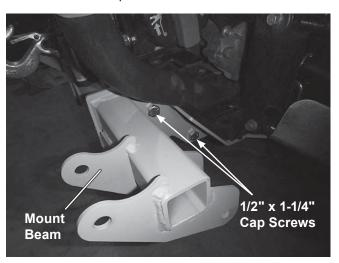
9. Verify that the mount beam is level from left to right and tighten the 1/2" fasteners according to the torque chart.
