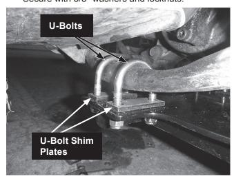
Tighten all fasteners according to the torque chart. Ensure that each U-bolt leg is tightened evenly.
