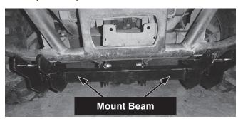
3. With the vehicle parked on a level surface, measure from the ground to the center of the rear hole in the mount beam. If this measurement is less than 9-1/2", installation of the front suspension lift kit is required.
