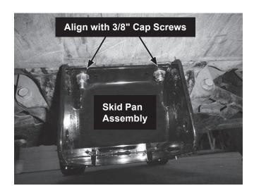
4. Place U-bolt shim plates in position on the top side of the skid pan assembly. Position two U-bolts on each side of the mount (four total), as shown. Check that the U-bolts have at least 1/4" clearance from any other vehicle components. Adjust the position forward or aft, as needed. Secure with 3/8" washers and locknuts.
