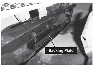
3. Position the mount's skid pan assembly in place against the bottom of the bumper as shown. Align the outer front holes in the assembly with the 3/8" cap screws installed in Step 2. Secure with 3/8" washers and locknuts. Do not tighten any fasteners at this time.
