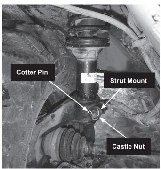
Remove the nuts securing the top of the strut to the vehicle body. It may be necessary to remove the heater (if equipped) to gain access to the top strut nuts.
