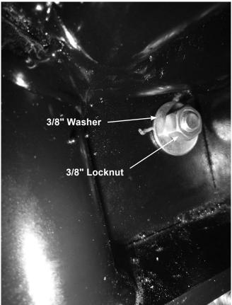
3. Install a 3/8" U-bolt on both sides of the vehicle, placing it over the frame tube and through the forward-most set of U-bolt holes. Secure with 3/8" locknuts, and hand tighten.
