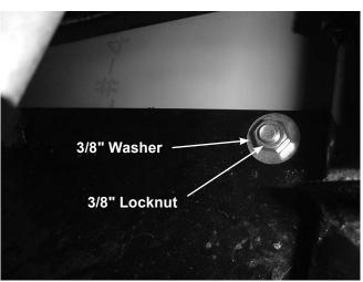
2. Install four 3/8" cap screws through the holes in the front of the skid plate assembly. Secure with a 3/8" washer and locknut, and hand tighten.
