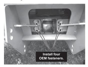
9. Keep the skid plate assembly level throughout this step. In order to maintain even pressure of the skid plate assembly against the frame tube, it is necessary to tighten each fastener incrementally in multiple passes, working from driver's side to passenger's side. At the final pass, tighten each fastener according to the torque chart. 10. To access the driver's side of the front gusset for the following step, turn the vehicle steering wheel all the way to the left.
