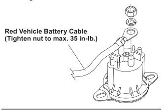
NOTE: Use dielectric grease on all electrical connections to prevent corrosion. Fill receptacles and lightly coat ring terminals before assembly.
