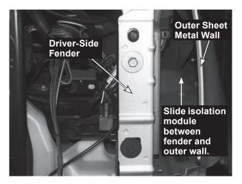
Install the isolation module on the inside of the driver-side fender using the supplied cable ties, reclosable fastener strips, and edging material as shown below.
