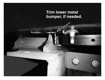
16. Notch the lower plastic section of the bumper to allow clearance for the U-brackets. Reattach the bumper using the original fasteners.
