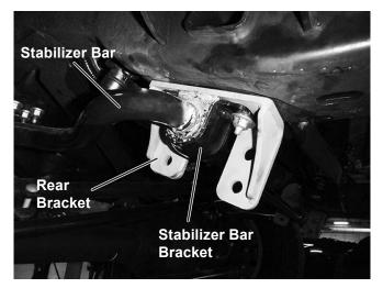
Position the passenger-side mount as shown. Insert two 1/2" x 2" cap screws through the mount holes against the inner frame surface. Secure with 1/2" locknuts and 1/2" washers on the inside of the frame.
