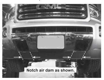
2. Remove the tow hook fasteners. Leave the tow hook in place. Position the passenger-side mount as shown below, with the inner surface of the mount against the tow hook.
