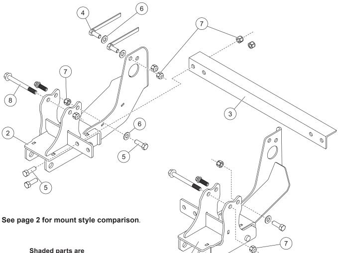
Shaded parts are original vehicle components.
