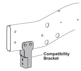
4. Install the mount by holding the front portion of the mount in place and securing with the previously removed bumper bracket bolt assembly.
