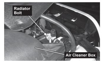
From underneath the truck, gently push the radiator up to clear the hooks that secure its lower section and move it rearward.
