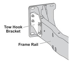
3. Remove the compatibility brackets from the frame, if so equipped (see illustration below). Save the brackets and hardware for the vehicle owner.
