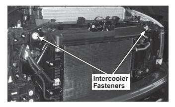
**On model year 2011 and later vehicles,** the radiator may need to be moved rearward to allow removal of the bumper bracket bolt. This is due to an added plastic and foam air-management structure on these vehicles. To move the radiator, remove the upper radiator bolts. The air cleaner box may have to be removed to access the passenger-side radiator bolt.
