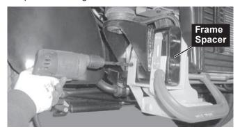
Use the hole in the bottom rear of the mount as a guide to drill a 17/32" hole through the bottom of the frame rail.
