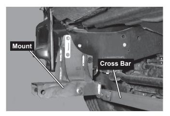
**On vehicles without compatibility brackets,** clamp the rear portion of the mount into position on the truck frame, making sure that the mount is tight against the bottom of the frame.
