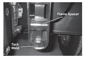
Insert one 1/2" x 1-1/2" cap screw with handle past the opening in the front frame spacer and into the truck frame. (Do not put a washer on this cap screw.) Fasten with a 1/2" locknut. Bend or trim cap screw handles after installation to avoid interference with vehicle components.
