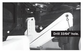
Locate the 1/2" x 1-1/4" cap screws with 18" handles. Insert the cap screw handles into the frame and insert the cap screws through the holes drilled in Step 6. Install 1/2" locknuts on the cap screws and finger tighten.
