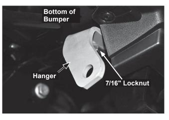
5. Position the skid plate assembly and the skid and splash pans as shown. Secure to the vehicle frame using the original OEM fasteners in the rearmost holes and upper holes. For upper holes, if reused fasteners do not fully engage the locknuts, use the 3/8" x 1-1/2" cap screws, 3/8" washers, and 3/8" locknuts provided.
