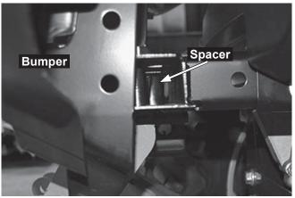
Place the driver-side hanger in position against the bottom of the bumper so that the 7/16" x 2-1/2" cap screws pass through the hanger holes. Secure with 7/16" locknuts and repeat on the passenger's side.
