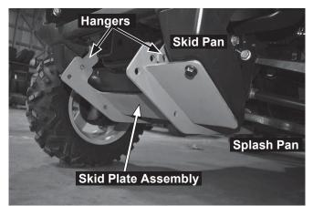
Secure the mounting beam to the skid plate assembly using four 1/2" x 1-1/4" cap screws and 1/2" locknuts. Tighten all fasteners according to the torque chart.
