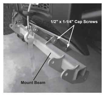
Measure the distance between the mount beam rear hole and the ground. If it exceeds 11-1/2", install the accessory Adapter Plates Kit (PN 77555) to ensure optimum plowing performance.
