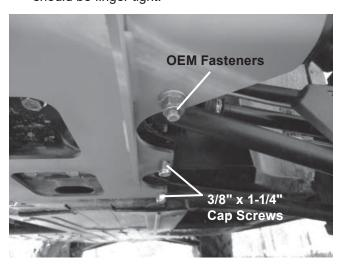
3. To install the driver-side bracket, position the driver-side bracket as shown.
