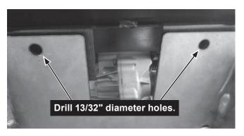
6. Secure the upper section of the skid pan assembly to the UTV frame by inserting 3/8" x 1-1/4" cap screws through the upper drilled holes, and securing with 3/8" washers and 3/8" locknuts behind the vehicle frame member. If needed, insert square washers between the frame and skid pan.
