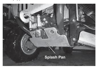
2. Remove and retain the two lower fasteners.
