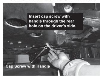
5. Insert a second cap screw with handle and washer, handle first, into the large hole located underneath and behind the front A-arm mount, with the handle toward the rear of the vehicle.
