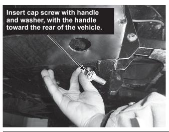
6. Insert both cap screws with handles through the corresponding holes as shown below.
