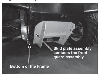
10. Tighten all hardware according to torque chart, including the UTV fasteners removed in Step 2.
