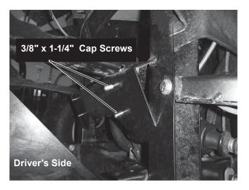
13. Insert the brackets over the 3/8" x 1-1/4" cap screws installed in Step 12. Secure with 3/8" washers and 3/8" locknuts. Hand tighten the locknuts. The photo below shows the correct pre-installation orientation.
