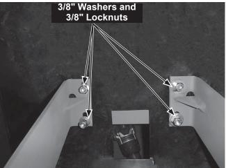
15. Tighten all hardware according to the torque chart, including the front guard fasteners if loosened in Step 2.
