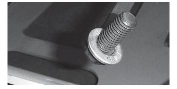
4. Insert one cap screw with handle and washer through the rear hole on driver's side, handle first, with the handle positioned toward the front of the vehicle.
