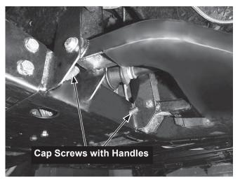
Place the skid plate assembly over the cap screws and secure with 1/2" washers and 1/2" locknuts.
