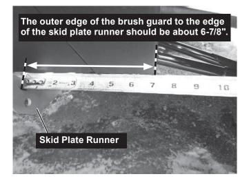
5. Measure the distance from the back edge of the front brush guard to the front edge of the skid plate as shown. Be sure that the distance is 3" on each side of the skid plate assembly. Adjust if needed.
