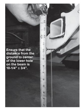
13. Measure the distance between the mount beam rear hole and the ground. If it exceeds 11-1/2", install the accessory Height Adapter Plate Kit (PN 77555) to ensure optimum plowing performance.
