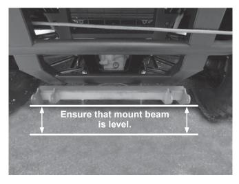
12. The distance from the ground to the lowest receiving hole on the mount beam should be approximately 10-1/4". Suspension adjustment may be necessary to achieve the proper ground clearance.
