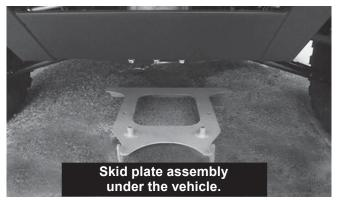
2. With the help of a second person, hold the skid plate assembly against the bottom of the frame. Center the skid plate from left to right. Be sure that the tail of the skid plate is between the two frame uprights. The passenger's side is shown in the picture below.
