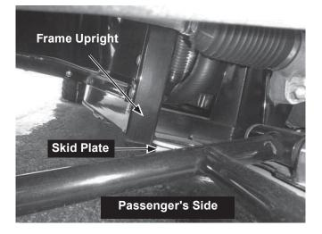
3. Tightly clamp the skid plate assembly to the vehicle on the both driver's and passenger's side using locking pliers in the location shown.
