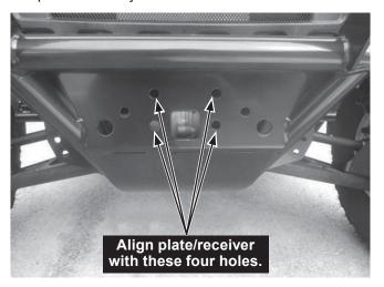
Insert a 1/2" x 1-1/2" cap screw into each of the holes. Secure with 1/2" washers and 1/2" locknuts. Hand tighten the locknuts.
