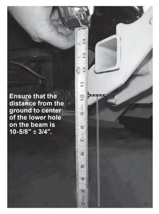
Measure the distance between the mount beam rear hole and the ground. If it exceeds 11-1/2", install the accessory Height Adapter Plate Kit (PN 77555) to ensure optimum plowing performance.
