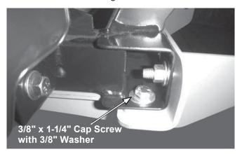
8. Tighten all hardware according to the torque chart, starting at the front of the vehicle. Recommended torque for the U-bolts is 30.8 ft-lb.
