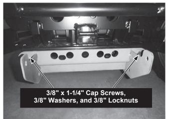
5. Trim plastic in rear as necessary to allow skid plate to contact the vehicle frame rails.
