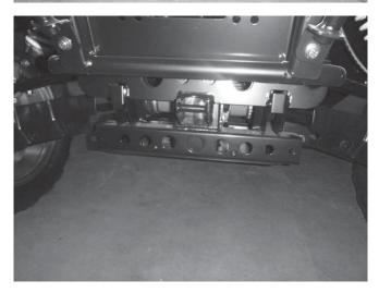
**For all Exmark, Toro, and 2014–15 Arctic Cat Models:** Remove the lower metal brush guard bolts; retain the fasteners for reinstallation.
