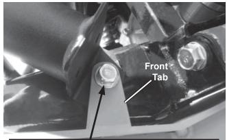
Align tab holes with holes on the vehicle. Install M10 x 1.25 x 30 cap screw on each side. 5. Clamp the rear of skid plate assembly to the vehicle frame.
