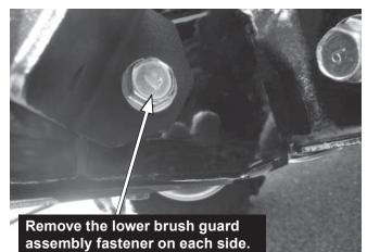
4. Place the front tabs of the skid plate assembly over the brush guard assembly, aligning the tab holes with the holes on the vehicle. Install an M10 x 1.25 x 30 cap screw on each side.
