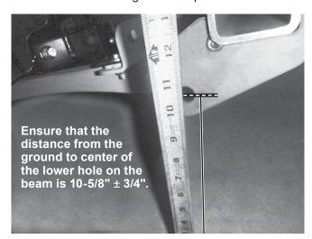
Measure the distance between the mount beam rear hole and the ground. If it exceeds 11-1/2", install the accessory Height Adapter Plate Kit (PN 77555) to ensure optimum plowing performance.
