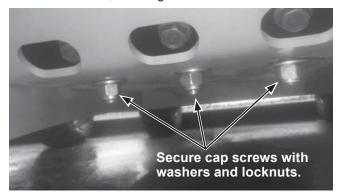
3. Insert a 1/2" x 1-1/4" cap screw through each of the four holes in the front of the skid plate assembly.
