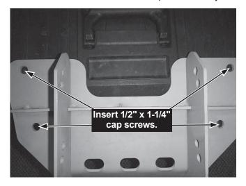
It may be necessary to loosen the winch mount to allow the fasteners to pass through the upper holes. Secure each cap screw with a 1/2" washer and 1/2" locknut; hand tighten.
