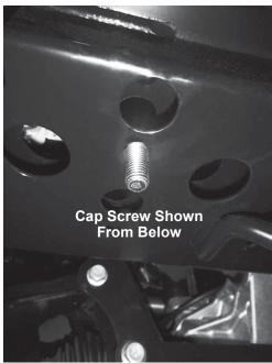
3. Install a hanger assembly over the 1/2" cap screw from Step 2. The cap screw should protrude through the middle hole of the hanger. Secure with a 1/2" locknut. Hand tighten the locknut.
