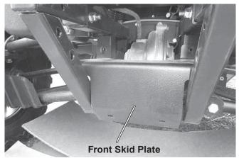
4. Remove the front skid plate. Retain for reinstallation if mount is removed.
