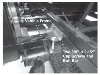
8. Starting at the front of the vehicle, tighten the fasteners installed in Steps 5–7 according to the torque chart.
