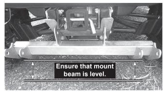
11. Measure the distance between the mount beam rear hole and the ground. If it exceeds 11-1/2", install the accessory Height Adapter Plate Kit (PN 77555) to ensure optimum plowing performance.
