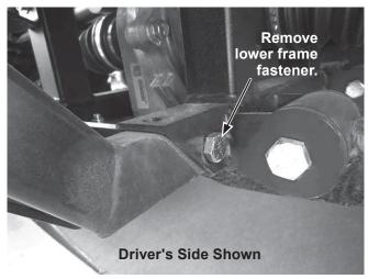
3. Remove the four fasteners holding the front skid plate in place. Save fasteners for reinstallation if mount is removed.
