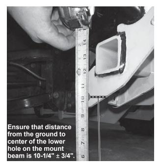
10. Check that the mount beam is level. Secure with four 1/2" locknuts. Tighten according to the torque chart.
