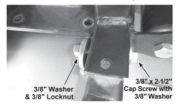
7. Insert two 3/8" x 2-1/2" cap screws through one of the bolt bars provided. Place the bolt bar over the vehicle frame and pass the fasteners through the skid plate assembly. Secure the cap screws with 3/8" locknuts; hand tighten. Repeat on the opposite side of the vehicle.
