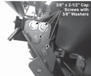
Place 3/8" washers on two 3/8" x 2-1/2" cap screws. Install the fasteners through the lower frame connection and the skid plate assembly. Secure with 3/8" washers and 3/8" locknuts; hand tighten.
