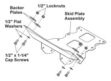
Secure each fastener with a backer plate and locknut.
