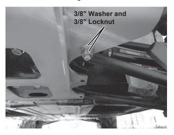
4. Place a 3/8" washer on each of two 3/8" x 1-3/4" cap screws. Install the cap screws through the remaining bottom holes. Secure with 3/8" washers and 3/8" locknuts. Hand tighten the fasteners.
