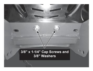
4. Fasten the driver-side bracket to the skid plate assembly using two 3/8" x 1-1/4" cap screws. A 3/8" washer must be used on both sides of the slotted hole. No washers are necessary on the bottom bracket/skid plate assembly hole. Secure with 3/8" locknuts. Hand tighten the fasteners.
