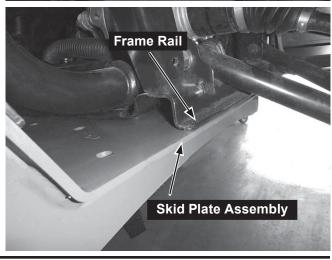
3. Push the skid plate assembly back against the front brush guard plate. Secure the front brush guard plate to the skid plate assembly using two 3/8" x 1-1/4" cap screws with 3/8" washers. Insert the fasteners through the middle slots as shown below. Secure with 3/8" washers and 3/8" locknuts. Hand tighten the fasteners.
