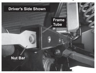
10. Place the driver-side bracket against the frame tube. Apply thread-locking compound to two 3/8" x 1-1/4" cap screws. Insert the two 3/8" fasteners through the bracket and frame tube. Thread the fasteners into the nut bar and hand tighten.
