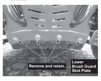
2. Place 3/8" washers on the two M10 x 45 cap screws. Place the skid plate assembly against the vehicle frame. Insert the M10 cap screws through the slotted holes in the skid plate assembly, up through the brush guard connector plate. Center the skid plate assembly and tighten fasteners until the skid plate assembly contacts the vehicle frame rails.
